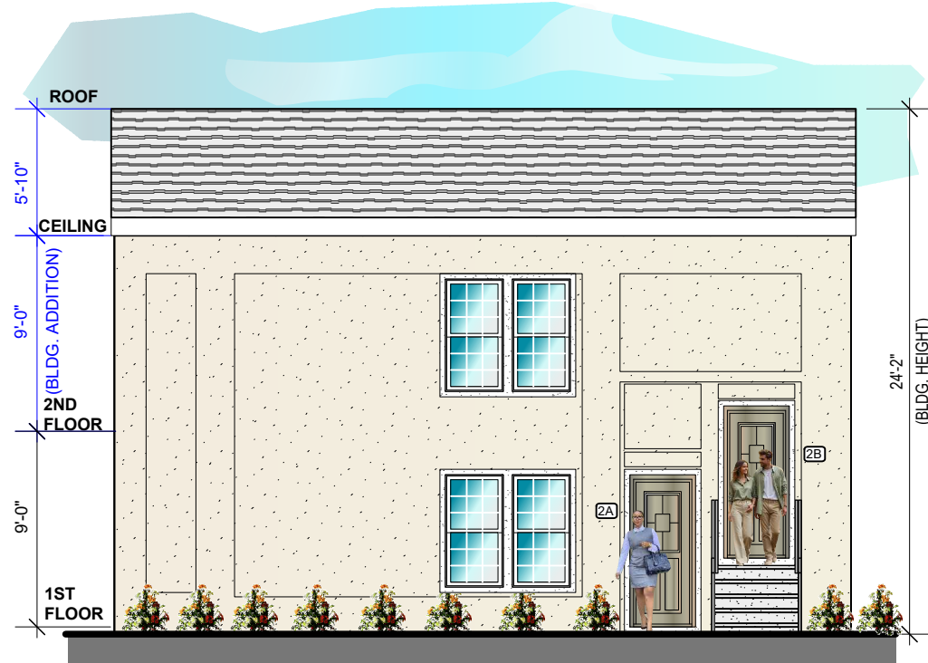
BLDG-2 PROPOSED FRONT ELEVATION (TUCKAHOE RD.) Scale: 1/8" = 1'-0"
