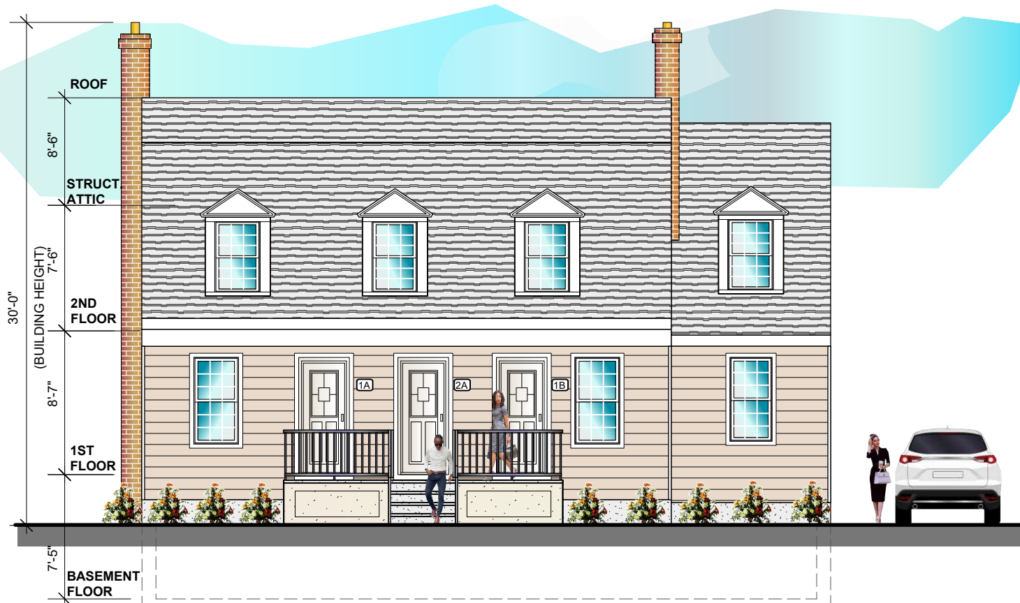
BLDG-1 PROPOSED FRONT ELEVATION (TUCKAHOE RD.) Scale: 1/8" = 1'-0"
