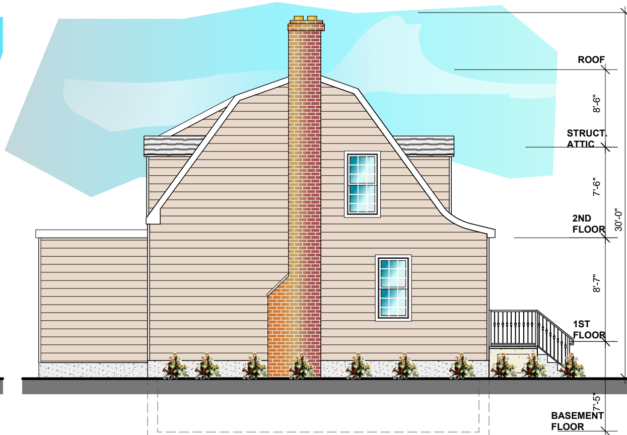
BLDG-1 PROPOSED LEFT SIDE ELEVATION Scale: 1/8" = 1'-0"
