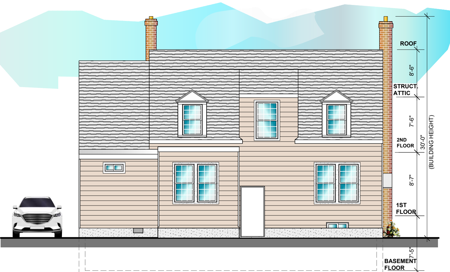
BLDG-1 PROPOSED REAR ELEVATION Scale: 1/8" = 1'-0"
